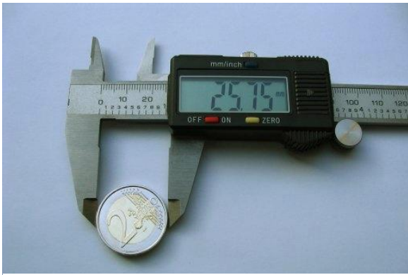
Fig. 9. The digital calliper.
